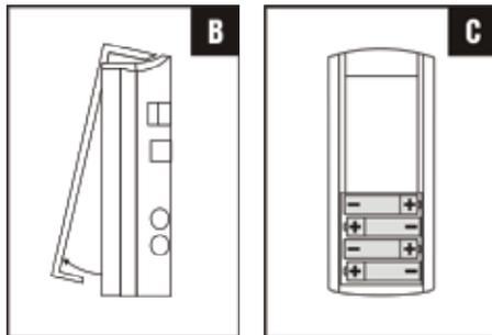
3. Replace the back cover and fix with screw.
